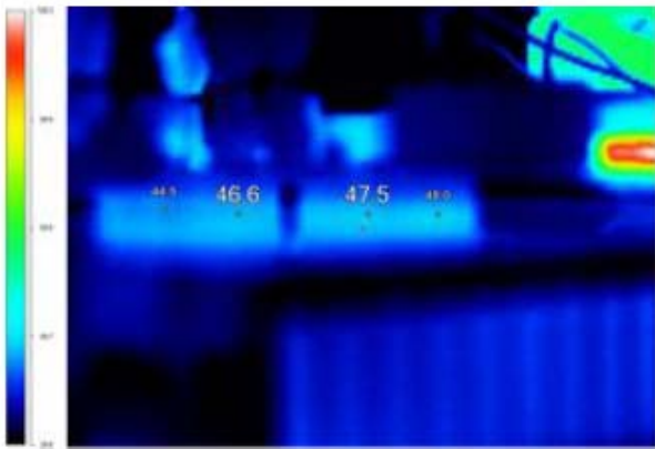
Fig. 12. Experimental results – thermal image of the tested circuit working in dual mode.
